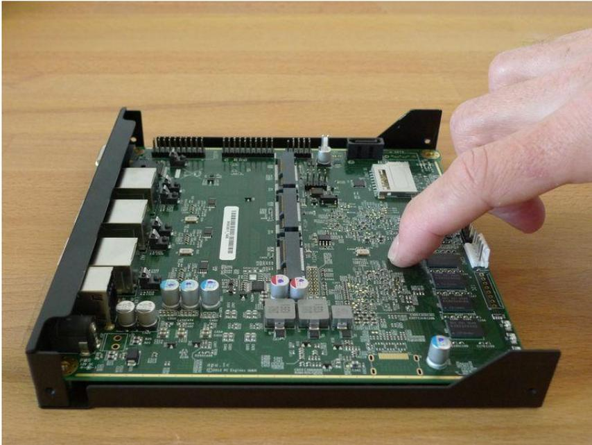
5. Insert SD-card or mSATA card to APU board. (Most of the kits have SD-card or mSATA SSD pre-installed.)
