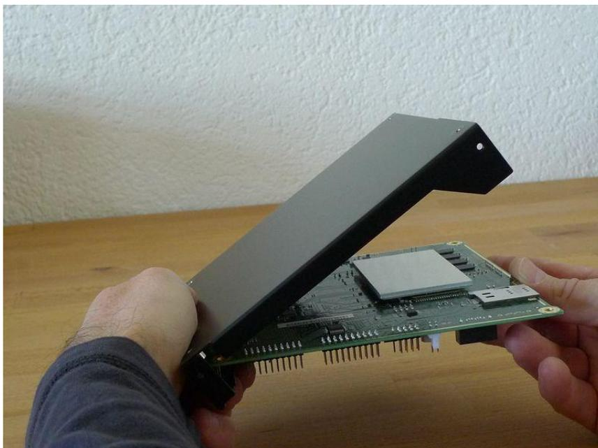
4. Turn around and carefully press down around CPU and heat sink to get good contact between enclosure and heat spreader. Then insert screws and hex nuts.
